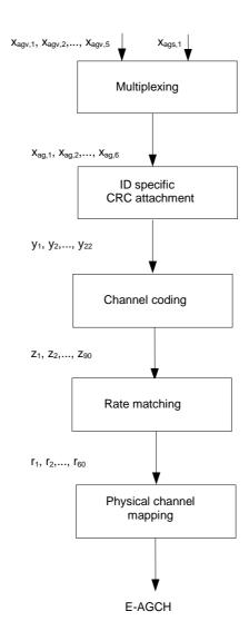
Figure 24: Coding for E-AGCH
